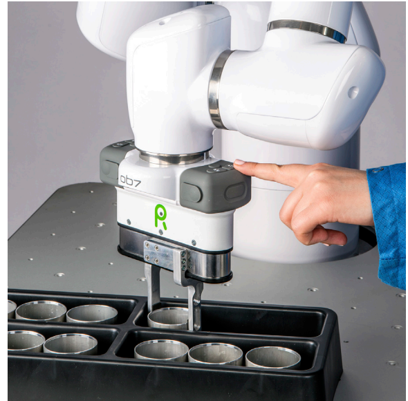
Press ◀▶ to open the gripper. and release the object.
