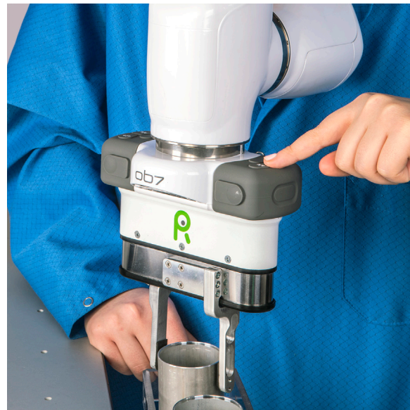
Press ►◄ to close the gripper.
