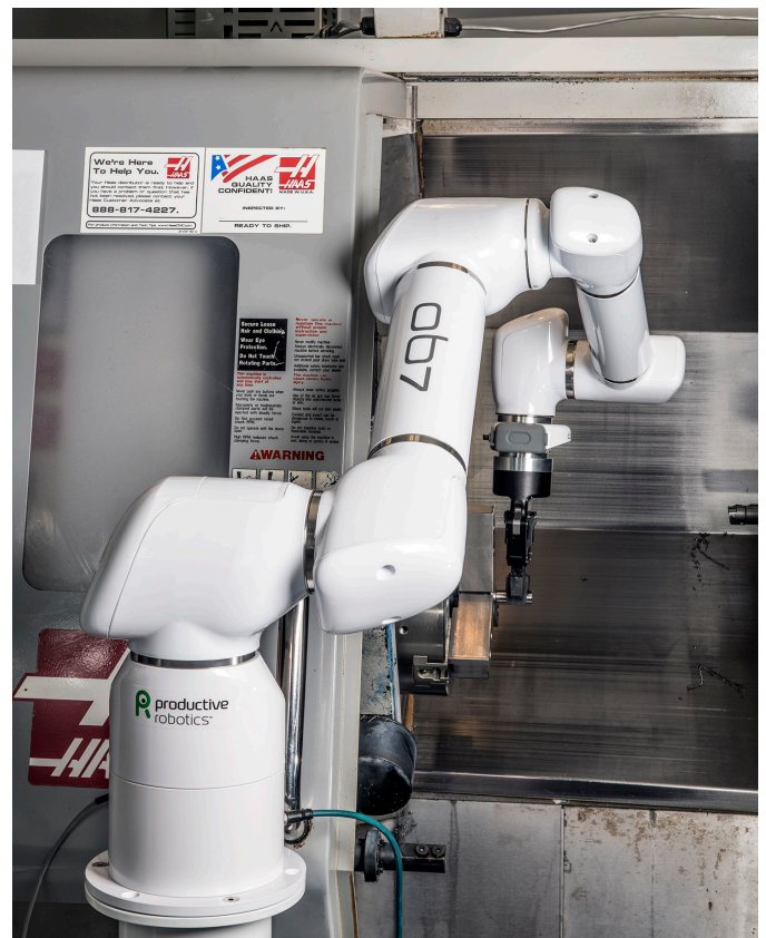
OB7's 7 joint arm has the capability to reach around objects.
