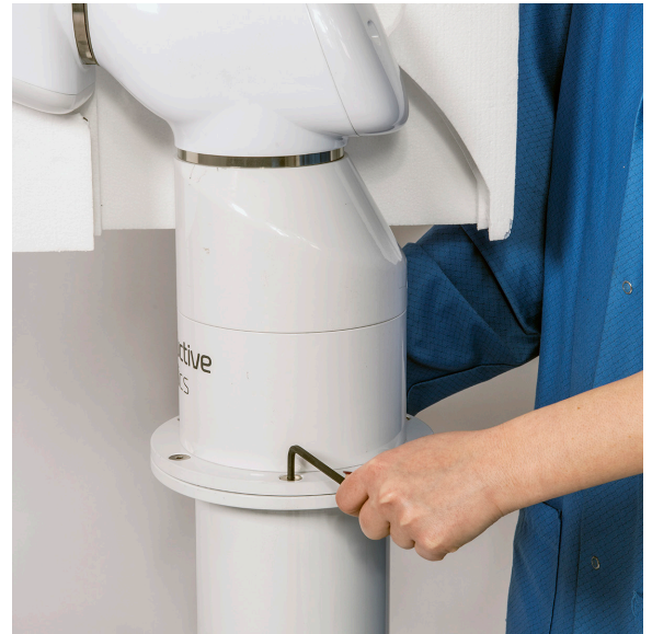
Tighten 8 mounting screws securely.
