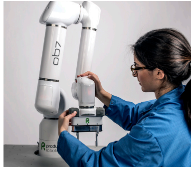
OB7 arms can be easily pushed and returned back to position.
