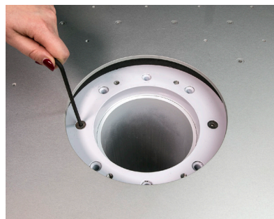
Using 4 M8 screws, attach the OB7 assembly table to the top of the stand column.
