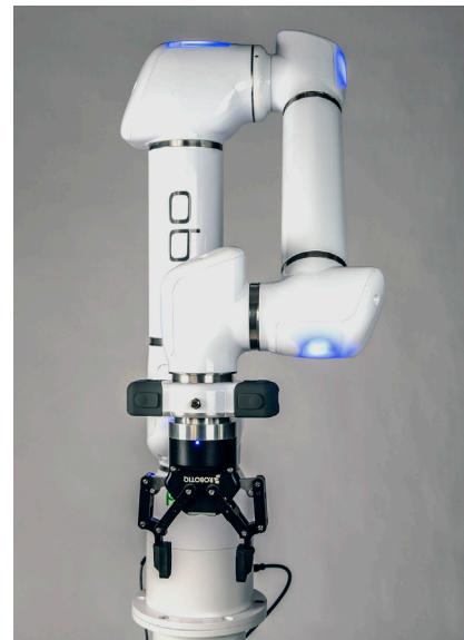
OB7 lights are blue, which means that OB7 is ready to Learn or Work.
