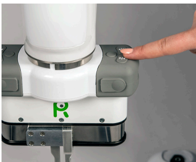
Press ►◄ to close the gripper.
