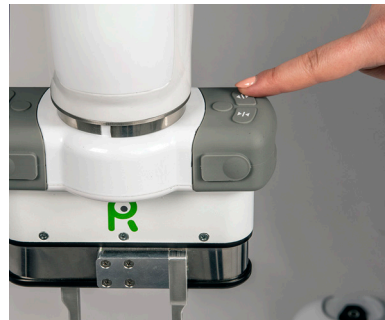
Press ◄► to open the gripper.
