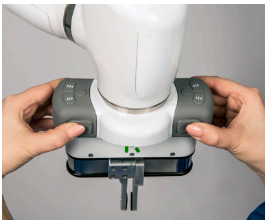
Use the control handle to move OB7 into a position.
